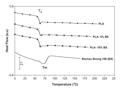
**Proof.** DSC measurements on various PLA samples with/without BS and of BS (second heating from -10 to 220 °C with a ramp of 10 °C/min).
