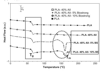
Figure 10. DSC measurements on various PLA samples with/without impact modifier (second heating from -10 to 220 °C with a ramp of 10 °C/min).
