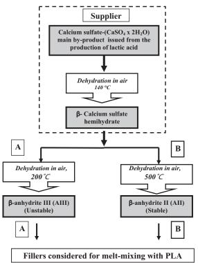
**Figure 1.**Schematic representation of the experimental routes considered for the preparation of the filler: (A)  $\beta$ -anhydrite III route; (B)  $\beta$ -anhydrite II route.
