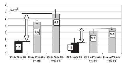
**Figure 7.**Notched impact strength (Isod) of PLA-AII compositions with/without impact modifier (ASTM D256-A, 3.46 m/s impact speed, hammer 0.668 kg).
