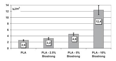
Notched impact strength (Izod) of various PLA compositions with/without BS (ASTM D256-A, 3.46 m/s impact speed, hammer 0.668 kg).
