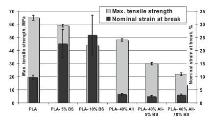
**Figure 8.**Tensile properties of PLA and PLA-BS compositions with/without AII filler (ASTM 638, specimens type V, v = 1 mm/min, distance between grips of 25.4 mm).
